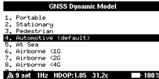
Access via **Settings > GNSS Dynamic Model**. Select the model that best matches your activity profile. Each mode adjusts the receiver's internal filters for optimal performance under different dynamics:
