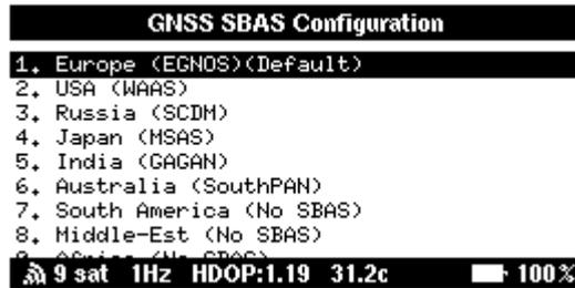
Access via **Settings > GNSS SBAS Configuration**. Select the regional Satellite-Based Augmentation System (SBAS) to enhance GNSS accuracy:
